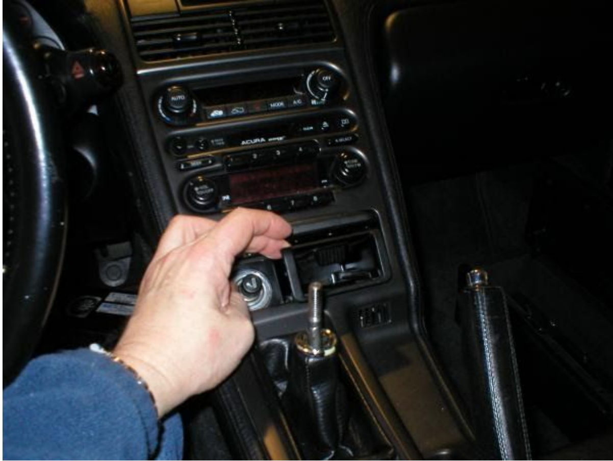
Lift the lid of the ashtray and remove the ashtray
