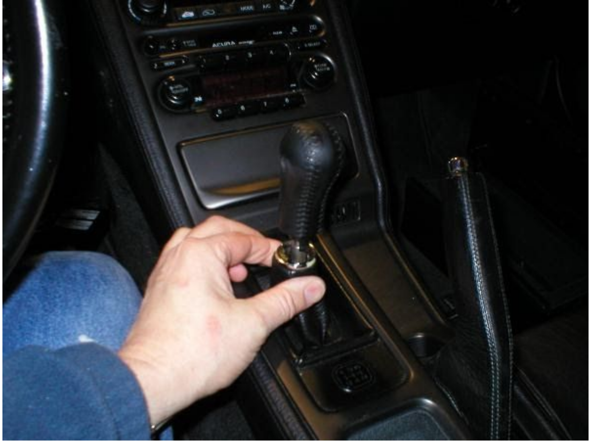
Pull the shift boot and chrome ring down and unscrew the shift knob
