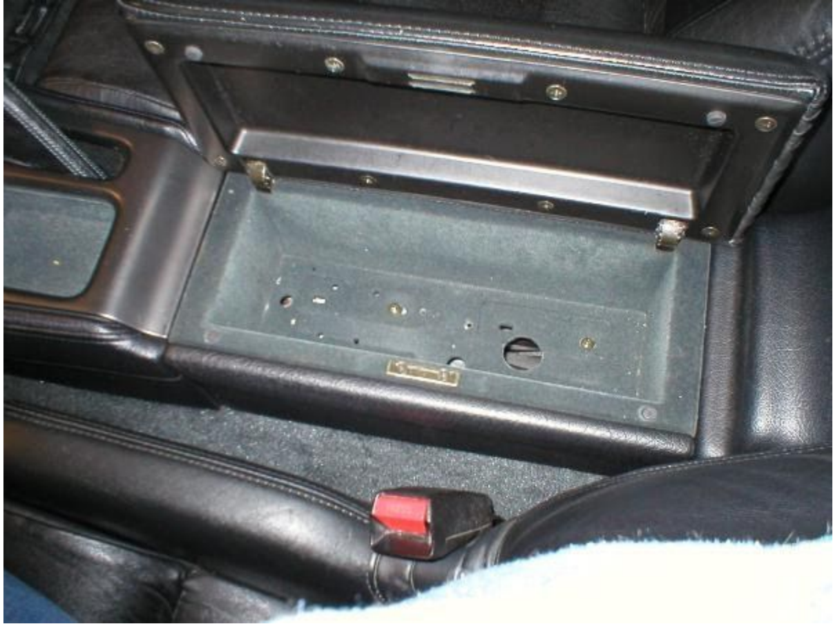
Remove the 4 screws holding the arm rest.
