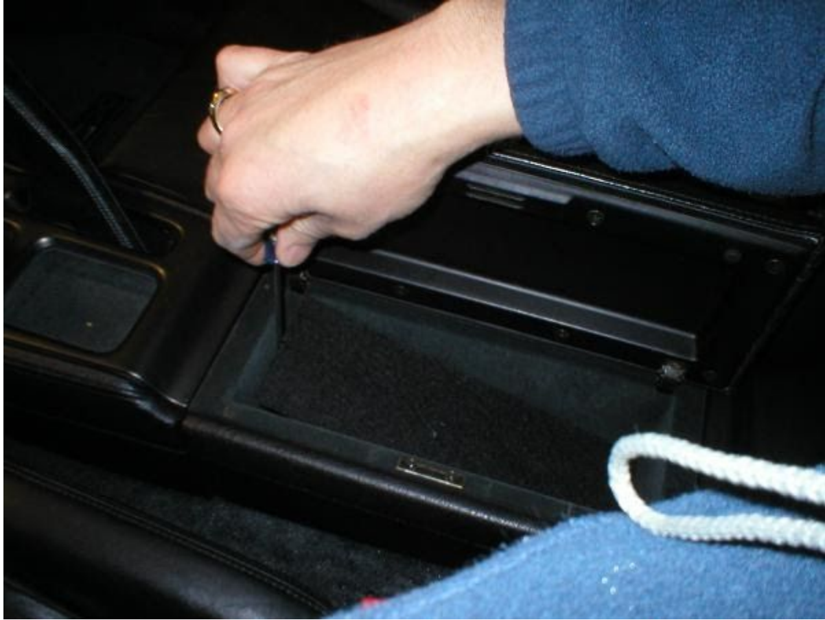
With a screw driver lift the false bottom of the arm rest
