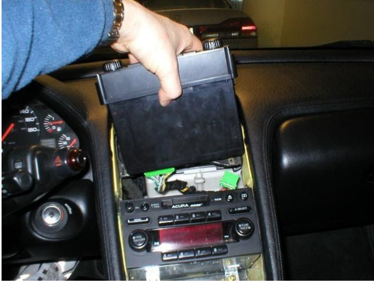
Lift out and disconnect the 2 connectors for the CCU
